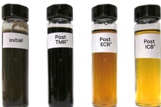
Fig. 7 Photos of EHC fluid sample before and after using TMR, ECR and ICB.
