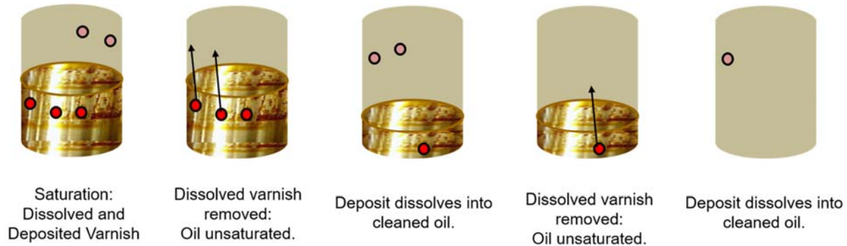
Figure 4: Complete Removal of Dissolved and Deposited Varnish by Ion Exchange Treatment.
