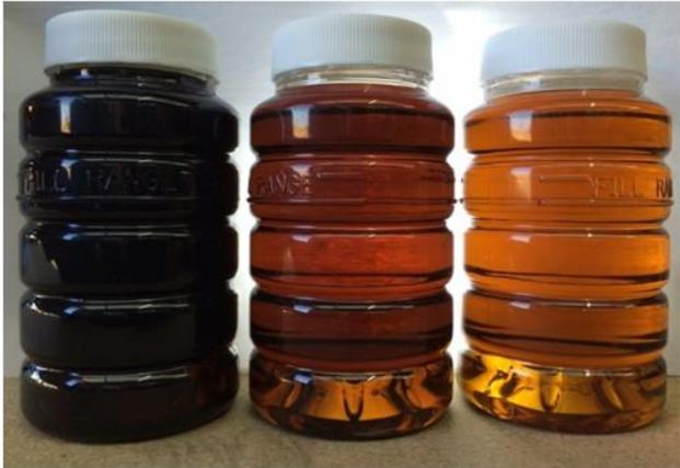
Figure 5: Improvement of EHC Fluid Appearance Following Electrostatic Filtration.
