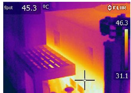
Fig. 7—Low operating fluid level in reservoir
