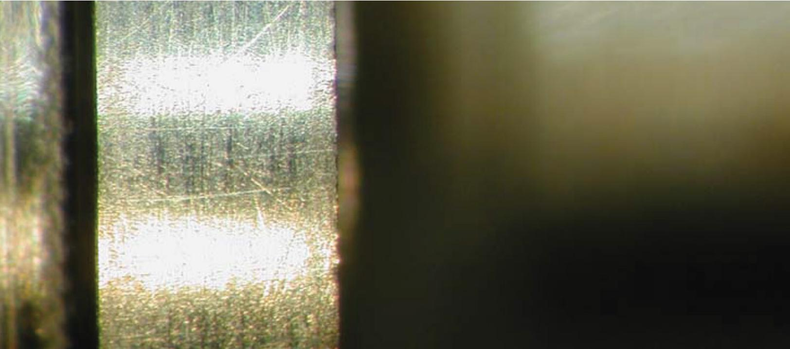
Photo of the pool null edge showing damage consistent with electron stream erosion.
