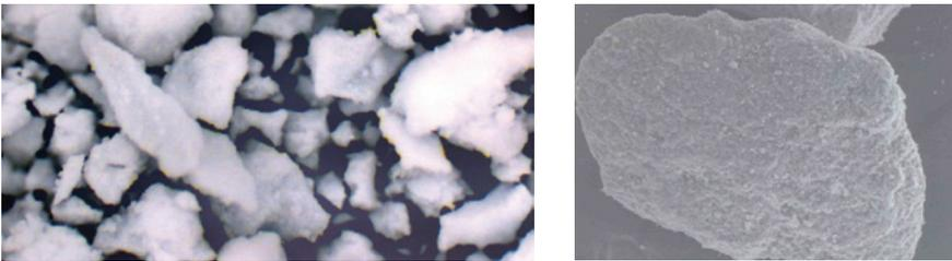
**Fig. 1**—Selexsorb GT alumina-based adsorbent (ABA) under 4x (left) and 120x (right) scanning electron microscopy (SEM) magnification showing abrasive aluminosilicate particles.
