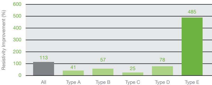
**Fig. 3**—Resistivity improvement differs between types of ion exchange media. EPT's proprietary ICB ion exchange media (Type E) provided the best average resistivity improvement.
