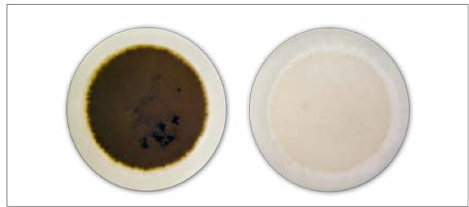
Fig. 1—Patch test results before and after ECR™ system.
