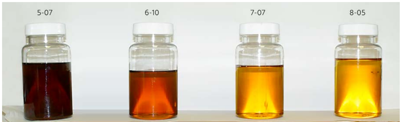
Fig. 2—Fluid clarity improvement over 3 months using an ECR™ system.
